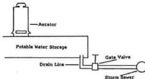
**FIGURE 1: Pipe-to-Pipe Cross Connection** A cross connection is created when the drain line is connected to the storm sewer.
