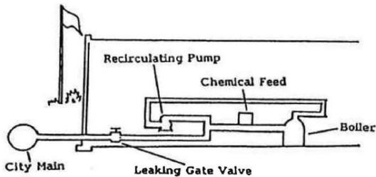
**FIGURE 3: Back Pressure Backflow.** *The recirculating pump for this boiler system will push water treated with corrosion inhibitors through the leaking gate valve into the city water supply.*
