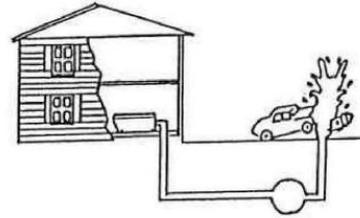
**FIGURE 4: Backsiphonage Backflow.** *The increased flow from the broken fire hydrant causes a vacuum in the service line and draws water from the bathtub through the submerged inlet into the distribution system.*
