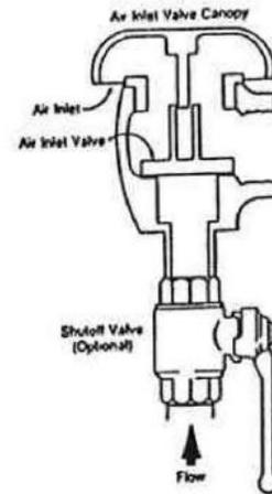
**FIGURE 6. Atmospheric Vacuum Breaker**
