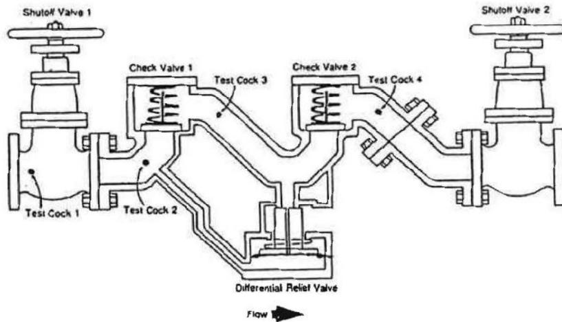
**FIGURE 9. Reduced Pressure Principle Backflow Preventer**
