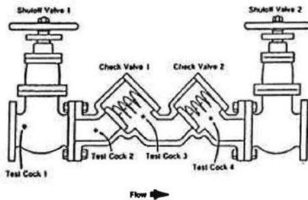
**FIGURE 8: Double Check Valve Assembly**
